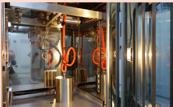
Cold Bend Cables Testing
